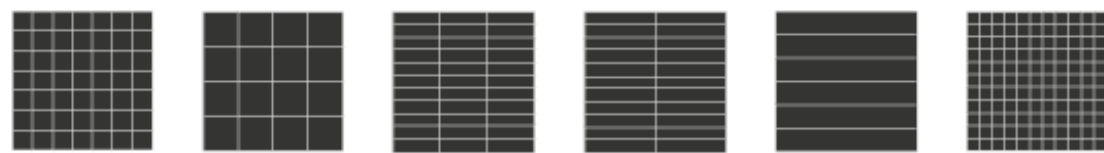
MOSAIC A 50x50 MOSAIC B 100x100 MOSAIC C 100x30 MOSAIC D 150x30 MOSAIC E 290x50 MOSAIC F 30x30
